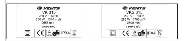
Design of rating label of other models is identical to the above except for type designation, rated power, ambient temperature, rpm and flow rate.
