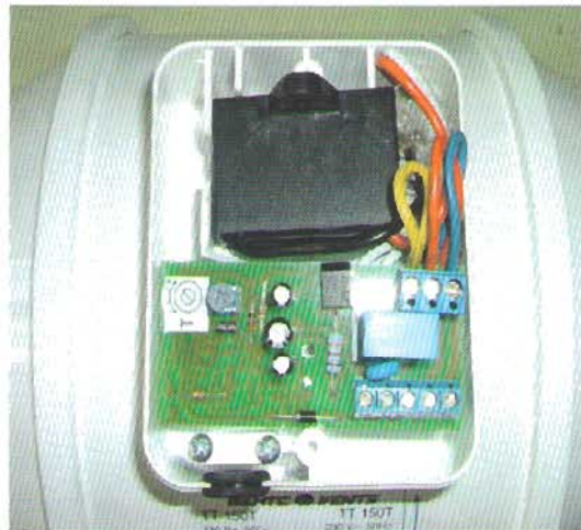
3. picture: TT 150T inside with PCB
